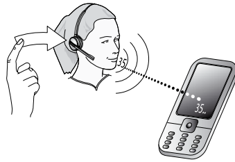
Figure 35: To use voice-activated dialing, tap the multifunction button and speak the appropriate voice tag.
