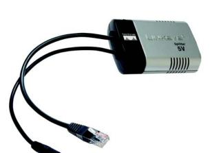
The Linksys 5 Volt Power Over Ethernet (POES5) Splitter lets you put your Linksys IP Phones almost anywhere, by removing the requirement of nearby power outlets. The POES5 sends power and VoIP over one Category 5 cable to your Linksys IP Phone. When it's time to add or relocate a phone, the POES5 can simplify your installation.
